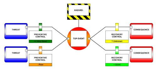
The BowTie diagram provides the visual representation of all the elements associated with a Hazard and the point at which control over the hazard is lost or compromised (Top Event). The left side of the BowTie diagram represents the various Threats that can lead to the loss of control represented by the Top Event as well as the Risk Controls necessary to *prevent* loss of control.
